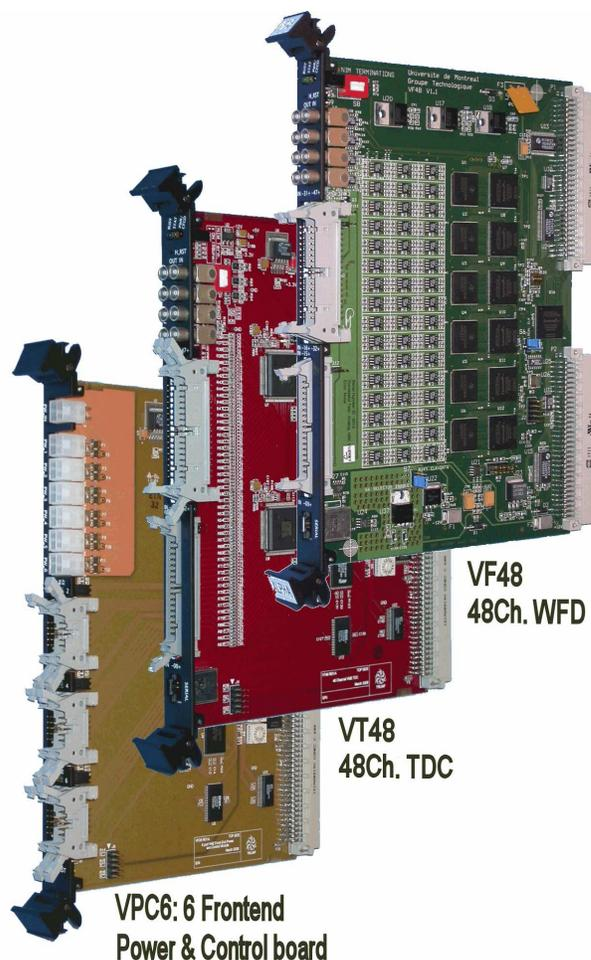
Fig. 1. VPC6, VT48, VF48 VME DAQ boards.
