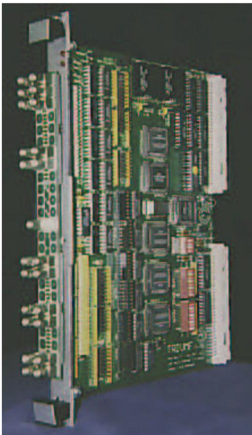
In keeping with the ongoing trend within the CHAOS group of translating CAMAC data acquisition elements to VME, we have designed and constructed a VME module to replace CAMAC Pattern-unit and Output-register functions. Notable features are:
