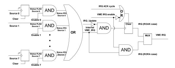
**Note:** Source 0 is shown as edge sensitive and source 1 as level sensitive input in the drawing above. Which interrupt sources are edge and level sensitive may vary from firmware implementation to firmware implementation.
