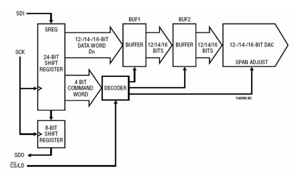
Figure 2.1: LTC1592 Block Diagram
