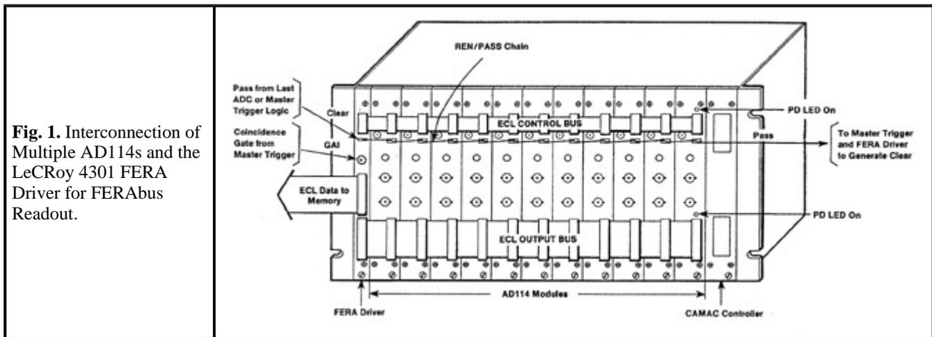
**Fig. 1.** Interconnection of Multiple AD114s and the LeCRoy 4301 FERA Driver for FERAbus Readout.
